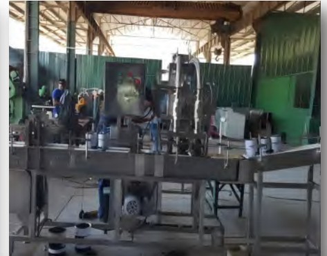
AUTOMATED HARDENER FILLING STATION FOR SOLID
