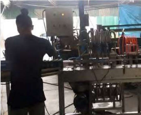
AUTOMATED HARDENER FILLING STATION 1
